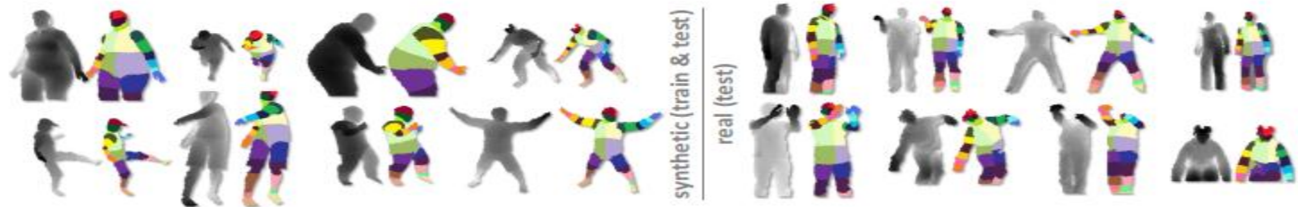
Figure 2. Synthetic and real data. Pairs of depth image and ground truth body parts. Note wide variety in pose, shape, clothing, and crop.
